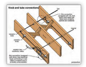
overheated in the past as a result of over-fusing, a poor connection or damaged cable. Often the wire becomes brittle in high heat areas, such as panels and junction boxes. In exposed areas, where inspection is easy, there is usually good air circulation and little heat build-up. The wires are least likely to be brittle in these areas.
