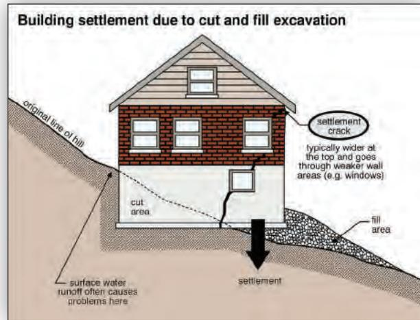
On sloping lots, large lateral earth thrust and hydrostatic pressure can be built up by the soil on the high side of the home.
