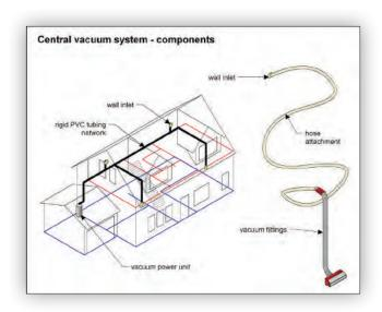
CANISTER The main canister usually has an on/off switch and may have a suction outlet as well. The exhaust may discharge directly from the canister or it may be piped through an exterior wall. Generally, units that do not have a filter must discharge to the exterior. Units equipped with a filter may discharge to the exterior or interior. The canister can be opened or removed to empty the unit. Some filters are self-cleaning while others require cleaning by the homeowner.
