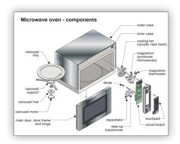
the oven disperses the microwaves into the oven as they leave the wave guide. In some units, a rotating tray on the oven bottom turns the food to ensure even cooking. A fan removes the heat generated by the food, and helps cool the magnetron.
