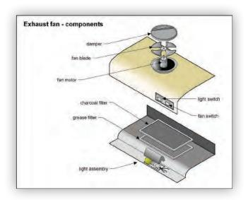
filters to help remove odors. In either case, filters are a regular maintenance item. Most mechanical filters are washable, and many can be cleaned in a dishwasher.
