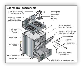
PILOT Traditionally, gas burners have been ignited with a pilot. In this system, a small flame (pilot) is always burning in the center of the range below the range top. When a burner is turned on, gas flows through a small tube towards the pilot. The pilot flame ignites the gas and the flame travels back up the open-ended tube to the burner, igniting the burner.
