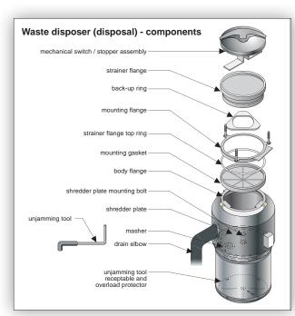
motor may stop and hum. The thermal overload protector cuts the power off after roughly 30 seconds. A jammed electric motor will eventually blow the fuse or trip the circuit breaker if the thermal overload does not trip.
